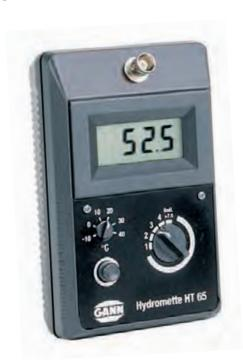
The HT 65 unit is an electronic wood moisture meter that uses the resistance principle of measurement for precisely measuring sawn timber (up to 180 mm in thickness), chipboards, veneers, wood chips, and similar bulk materials. The unit is used for individual measurements before and after processing.
