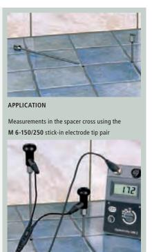
M 6 stick-in electrodes or M 20 drive-in electrode to be used in conjunction with the following units:
