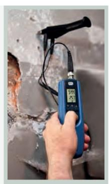
APPLICATION Measurement of plaster moisture using an M 20 electrode
