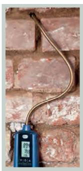
APPLICATION The flexible sensor pipe can be used to easily and conveniently carry out measurements in places that are difficult to access.
