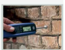
APPLICATION It is of importance how the unit is held while measuring: The BL Compact B 2 unit should be held at the rear part of the unit and applied to the material to be measured in a 90° angle.
