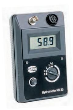
The HB 30 unit is an electronic wood and structural moisture meter that uses the resistance principle of measurement for precisely measuring sawn timber (up to 180 mm in thickness), chipboards, parquet, and set building materials.
